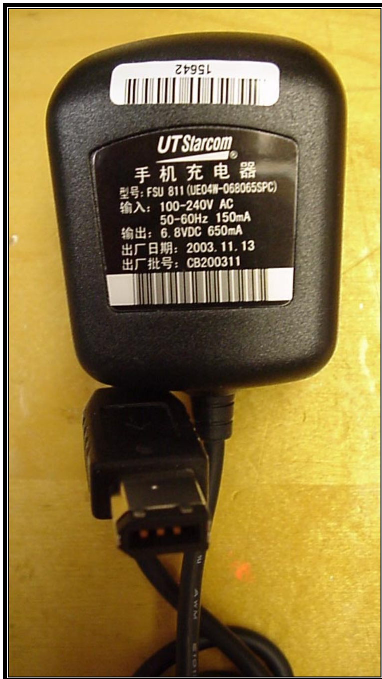
PHOTOGRAPH 22: 6.8 V DC POWER SUPPLY
