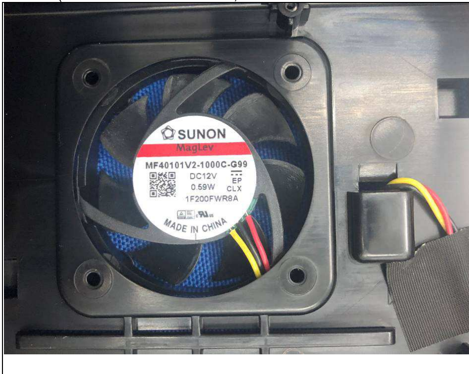
COOLING FAN 1 (MF40101V2-1000C-G99)
