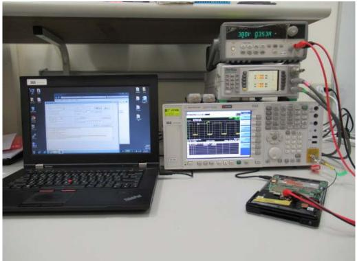
**Conducted Setup Photo (Measurement at Antenna Port)**
