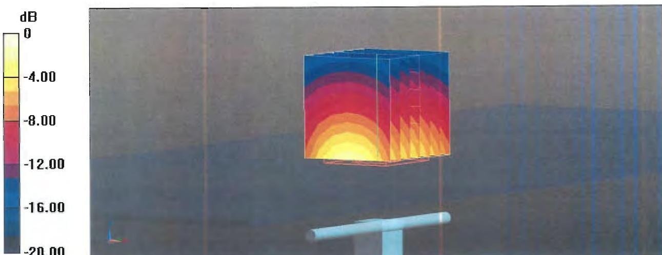
$$0 \text{ dB} = 15.7 \text{ W/kg} = 11.96 \text{ dBW/kg}$$
