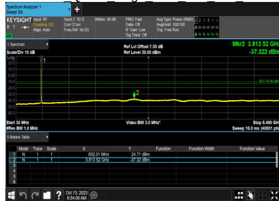
N5(10M)_DFT-s- OFDM QPSK Edge 1RB Left Mid CH
