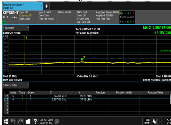
N5(5M)_DFT-s- OFDM BPSK Edge 1RB Left Low CH
