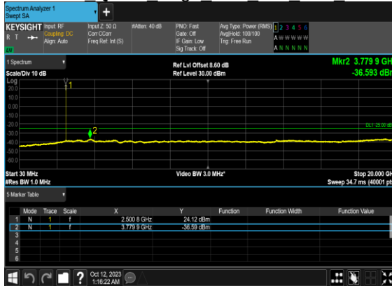
N7(5M)_DFT-s- OFDM QPSK Edge 1RB Left Low CH
