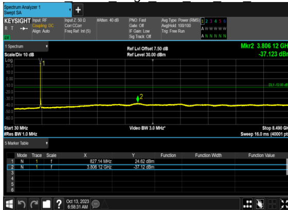
N5(20M)_DFT-s-OFDM BPSK Edge 1RB Left Mid CH
