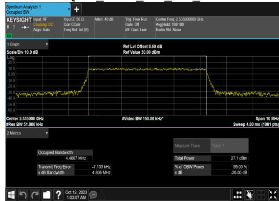
N7(5M)_CP-OFDM_256 QAM Outer Full Mid CH
