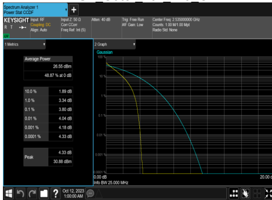
N7(20M)_DFT-s-OFDM_PI_2-BPSK Outer Full Mid CH
