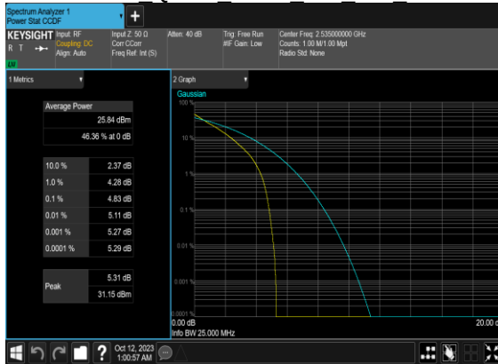
N7(20M)_DFT-s-OFDM QPSK Outer Full Mid CH
