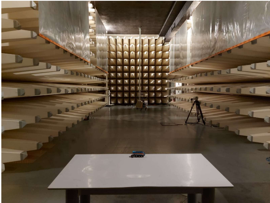
Set-up for Radiated Emission (Model: 3971)
