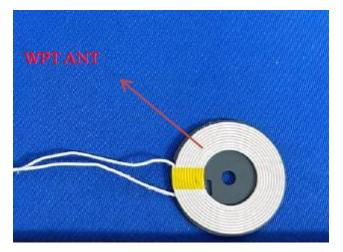
Antenna transmission frequency: 110.1kHz - 205kHz Antenna type: Coil antenna
