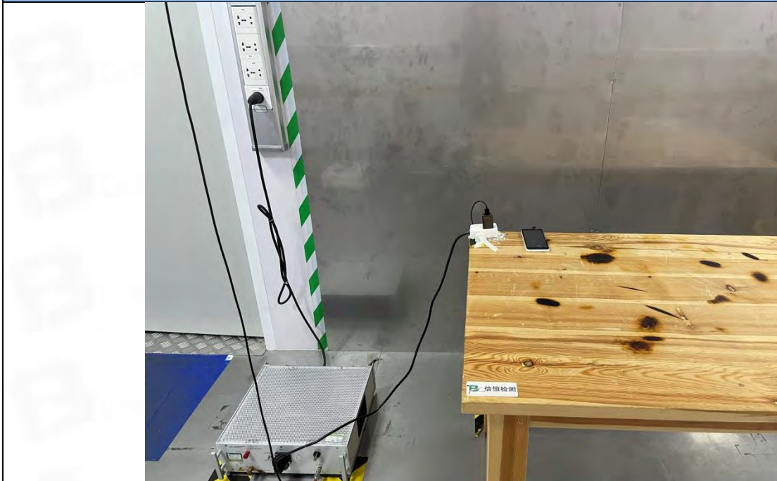
Conducted Emission at AC power line
