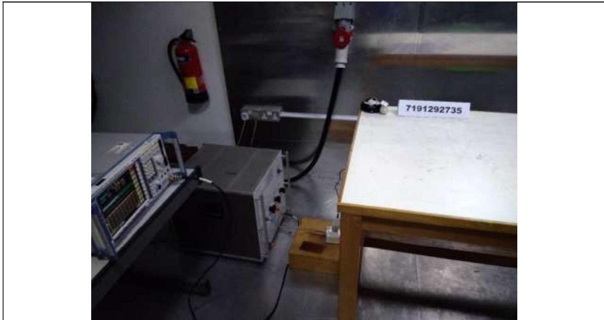
Conducted Emissions Test Setup (Front View)
