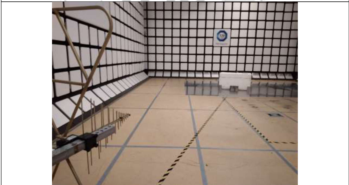
Radiated Emissions (Spurious Emissions Inclusive Restricted Bands Requirement) Test Setup (Rear View)
