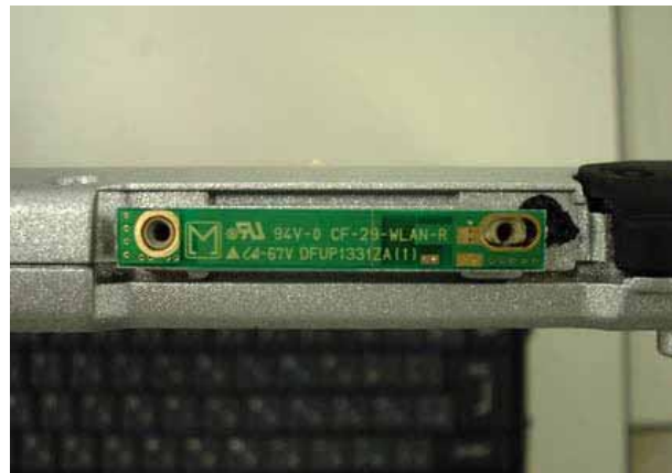
Main TX/RX Antenna View
