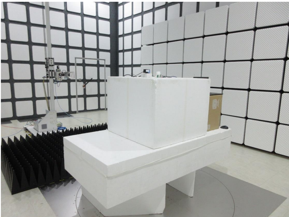
Description: Radiated Emission Test Setup for 1GHz~18GHz
