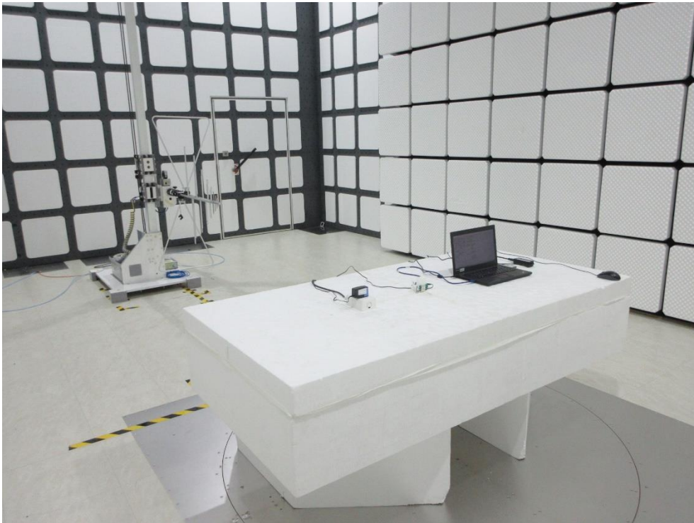
Description: Radiated Emission Test Setup for 1GHz~18GHz
