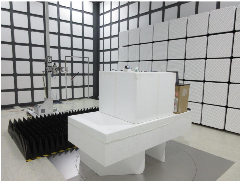
Description: Radiated Emission Test Setup for 1GHz~18GHz
