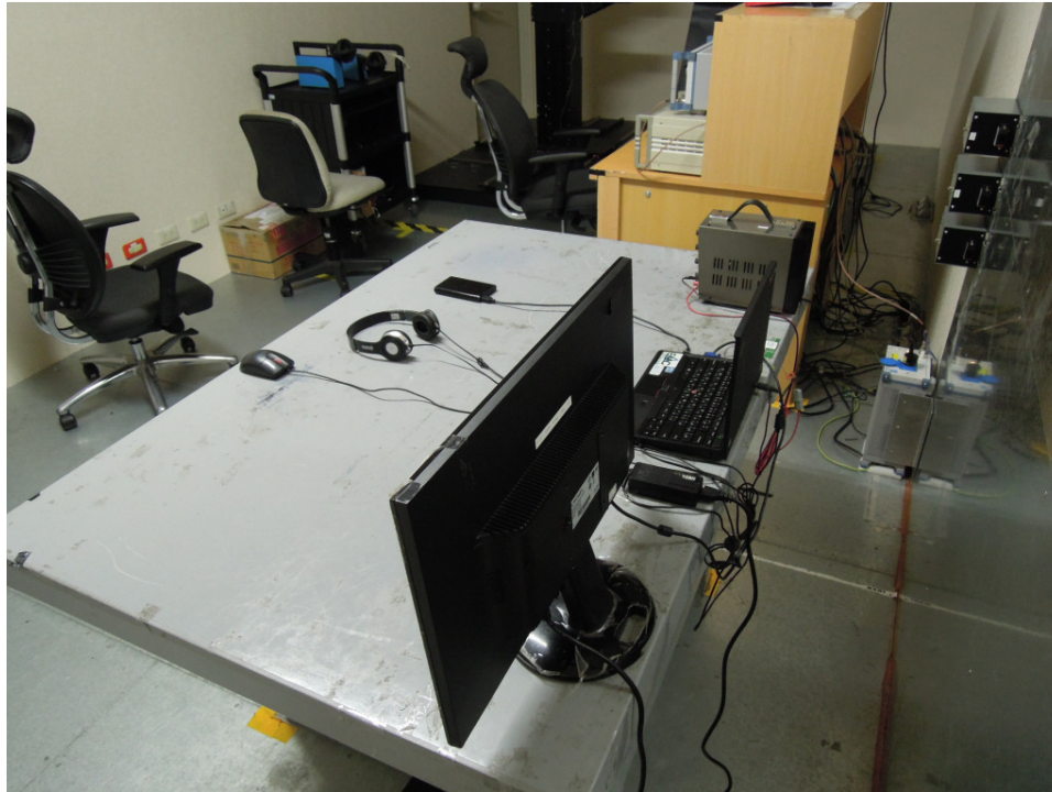
Photograph 7: Set-up for Mains Conducted testing (Back View)
