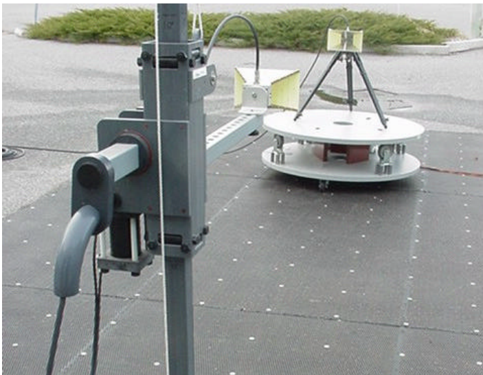
Signal Substitution Test Setup Photograph - Horn Antenna
