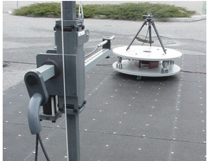
Signal Substitution Test Setup Photograph - Dipole Antenna
