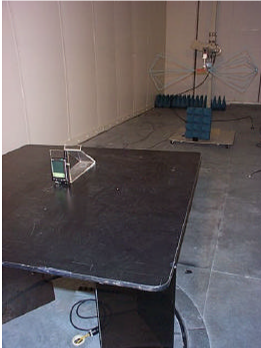
Palm V and WaveNet DWV 100D PDA Wireless modem Testing for Spurious Emissions from Transmitter Frequency Range: 30 MHz – 200 MHz
