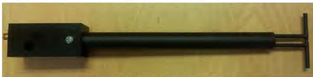
Figure 1 – MVG COMOSAR Validation Dipole
