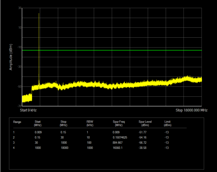
Band4 16QAM BW=10MHz Channel=20350 RB Size=1 Position=#0
