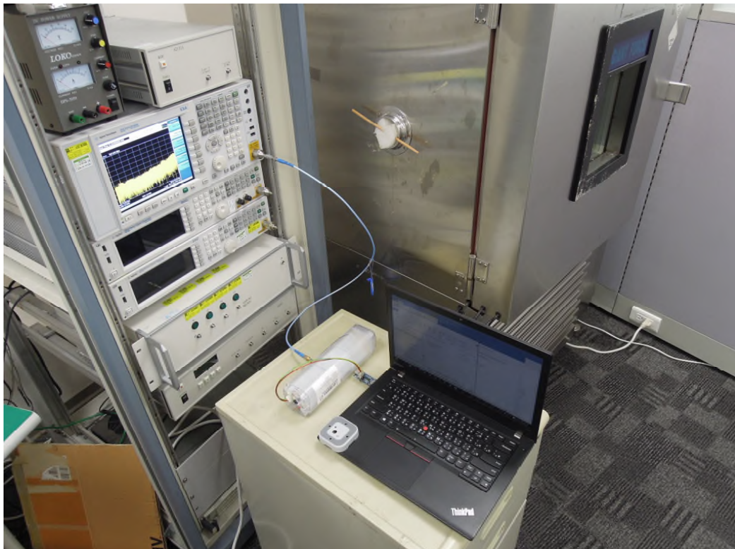
Photograph 4: Set-up for Conducted testing
