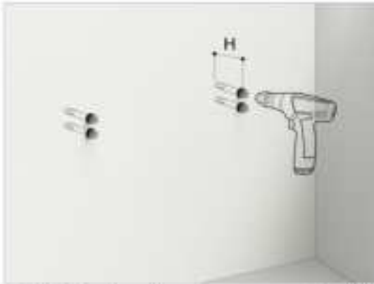
• Drill at the four sites using a percussion drill and embed 4x \varnothing 8 plastic expansion pipes.
