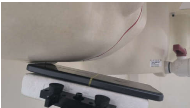
Right Tilted, Test Separation 0 mm
