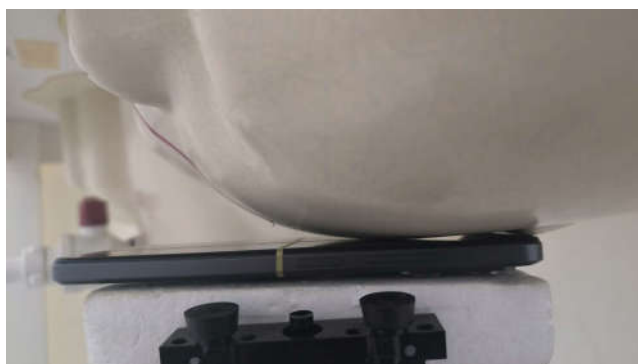
Left Cheek, Test Separation 0 mm
