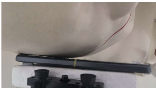
Right Cheek, Test Separation 0 mm
