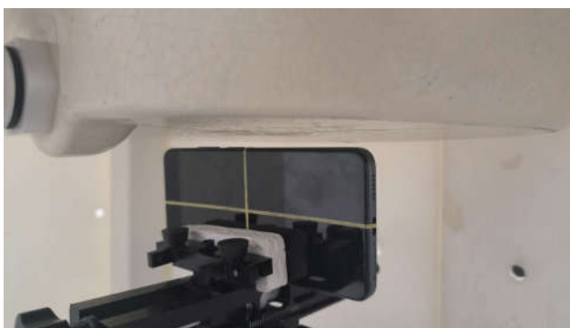
Right Side, Test Separation 10 mm
