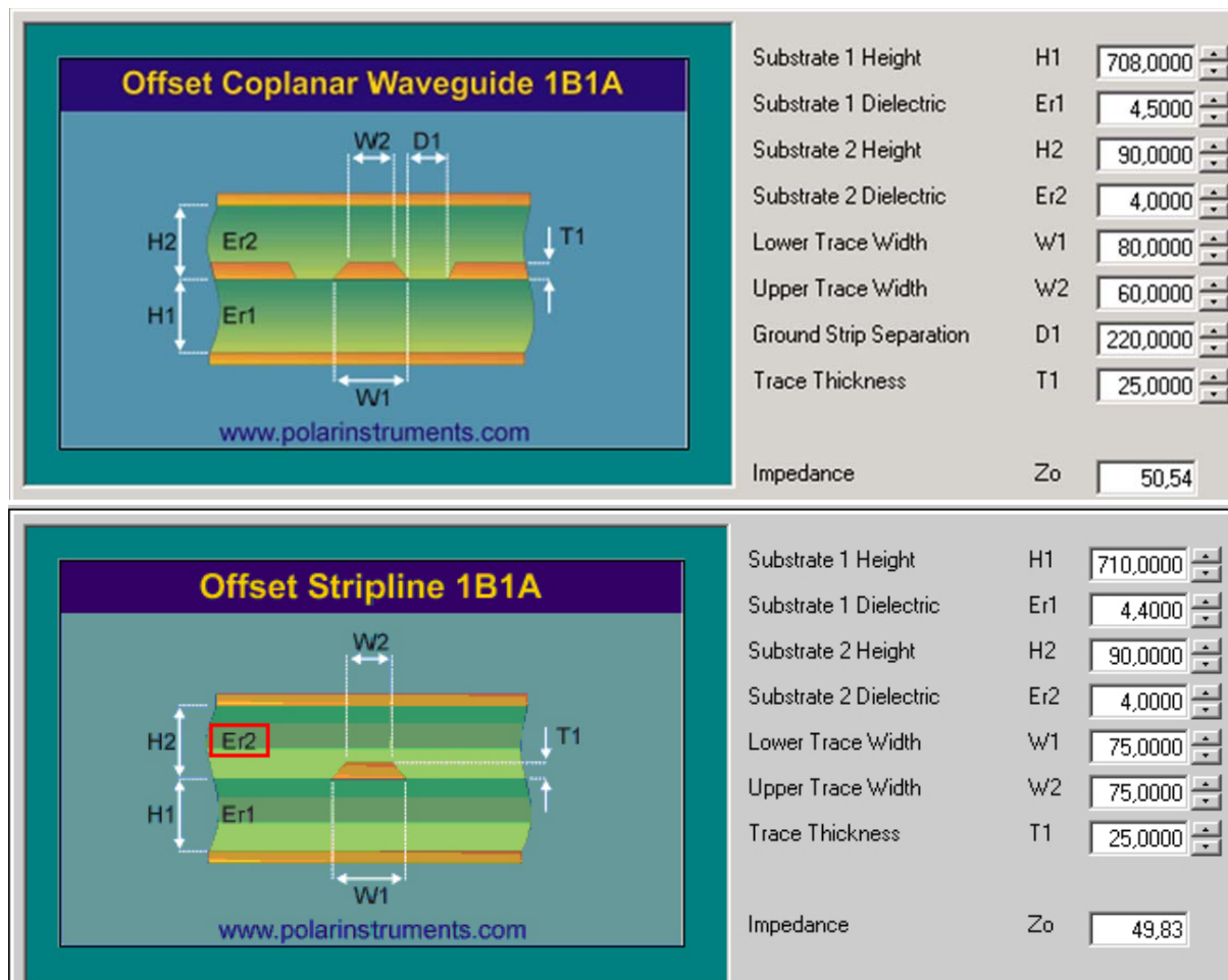
Figure 7: Embedded Stripline line arrangement
