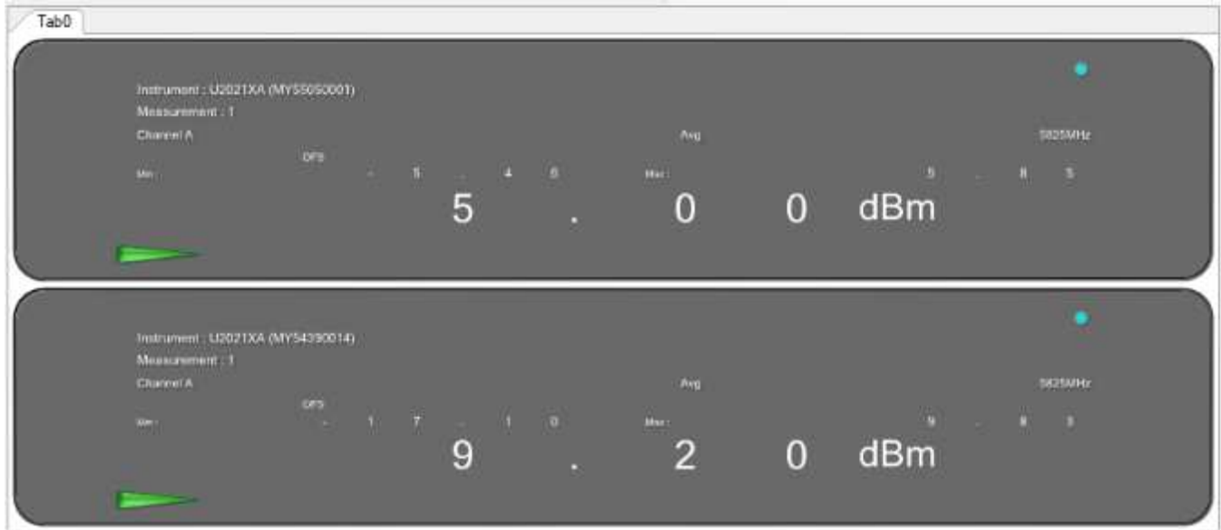
Figure 355: Maximum Conducted Output power measured at Ch.0 & Ch.1
