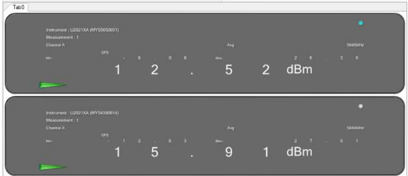
Figure 352: Maximum Conducted Output power measured at Ch.0 & Ch.1
