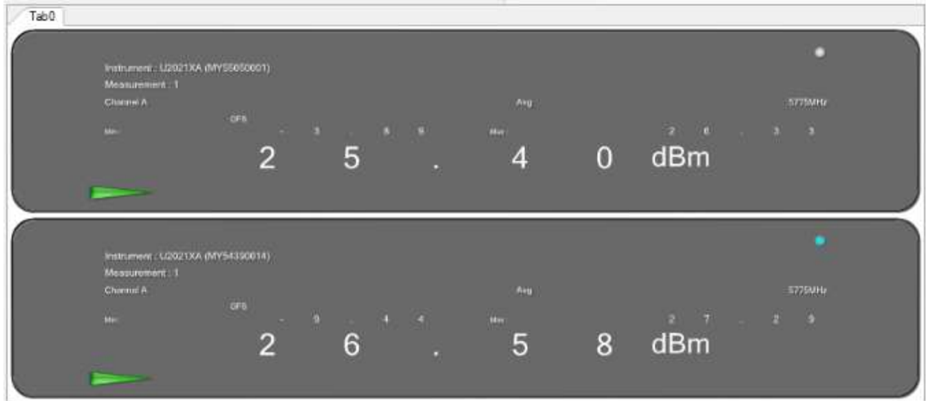
Figure 345: Maximum Conducted Output power measured at Ch.0 & Ch.1
