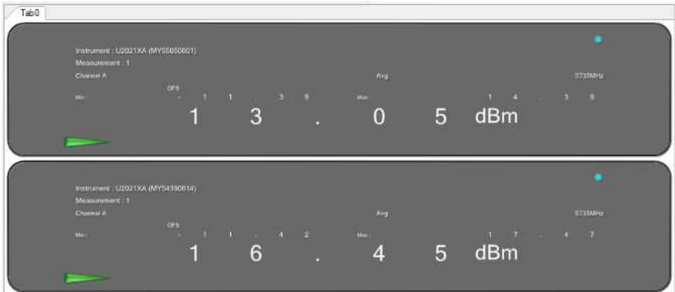
Figure 350: Maximum Conducted Output power measured at Ch.0 & Ch.1
