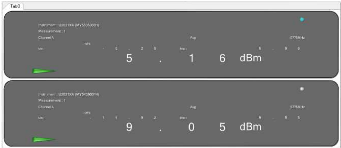
Figure 357: Maximum Conducted Output power measured at Ch.0 & Ch.1
