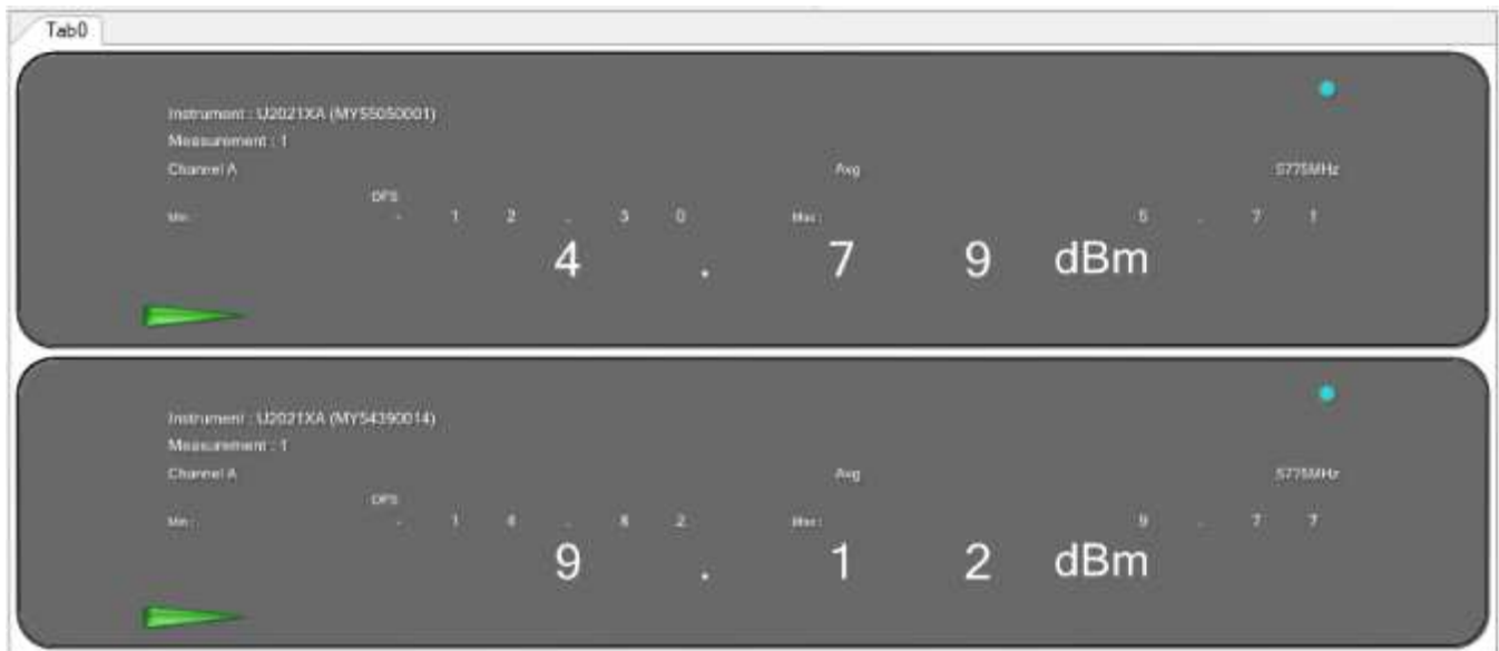
Figure 354: Maximum Conducted Output power measured at Ch.0 & Ch.1
