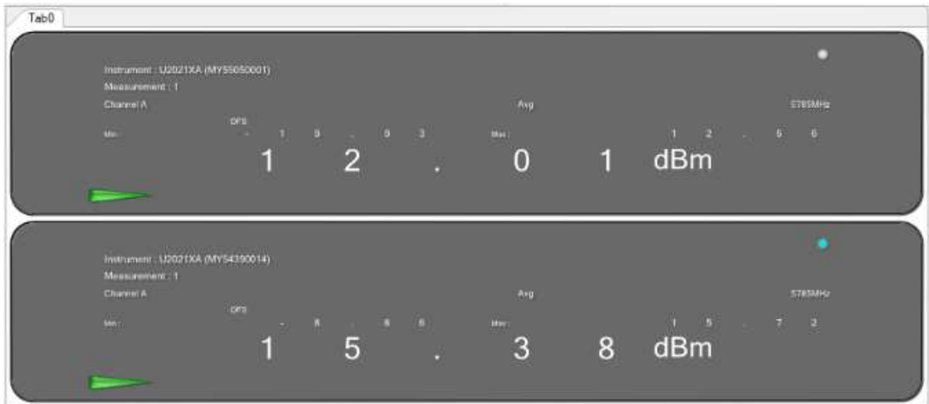
Figure 348: Maximum Conducted Output power measured at Ch.0 & Ch.1
