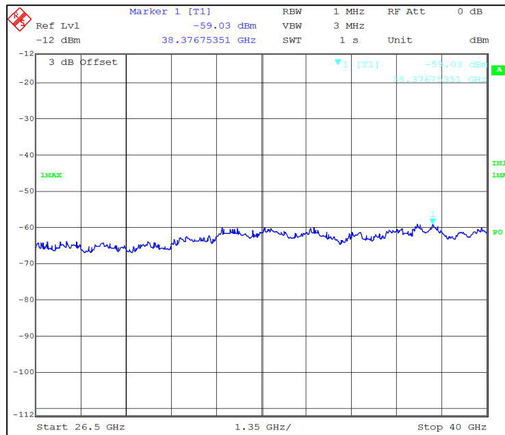
Figure 308: Emission measured with Peak Detector from 26.5GHz to 40GHz at Ch. 1
