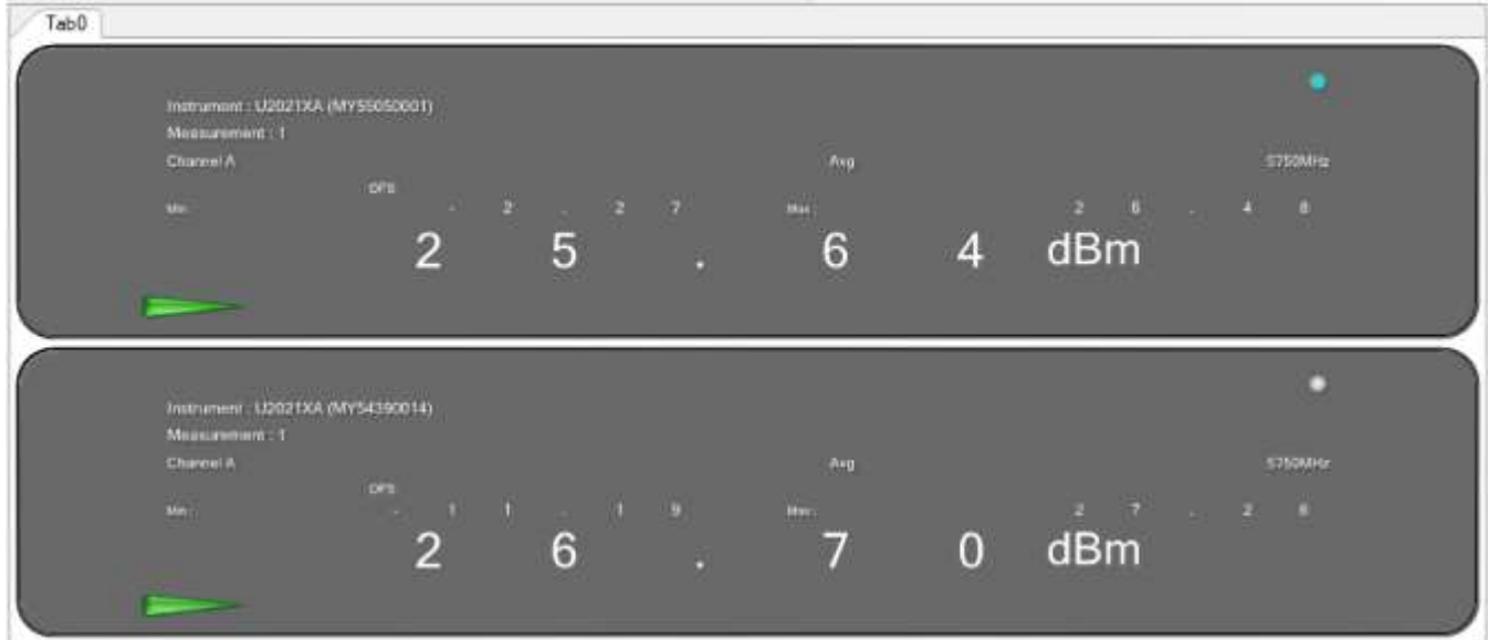
Figure 341: Maximum Conducted Output power measured at Ch.0 & Ch.1
