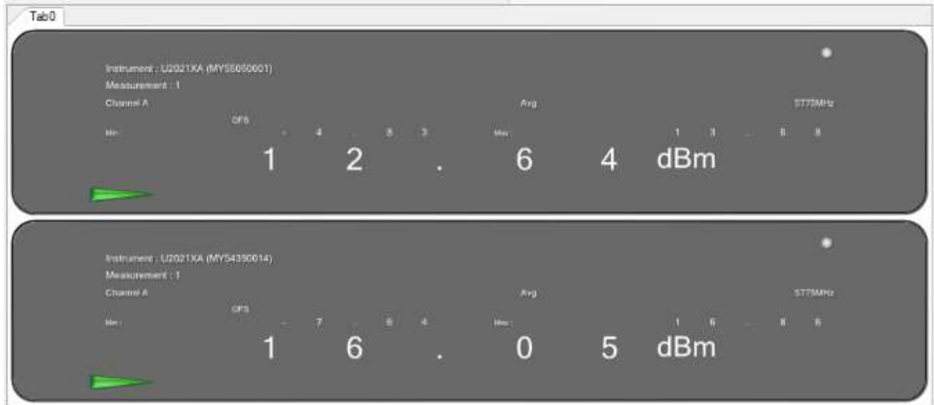
Figure 351: Maximum Conducted Output power measured at Ch.0 & Ch.1
