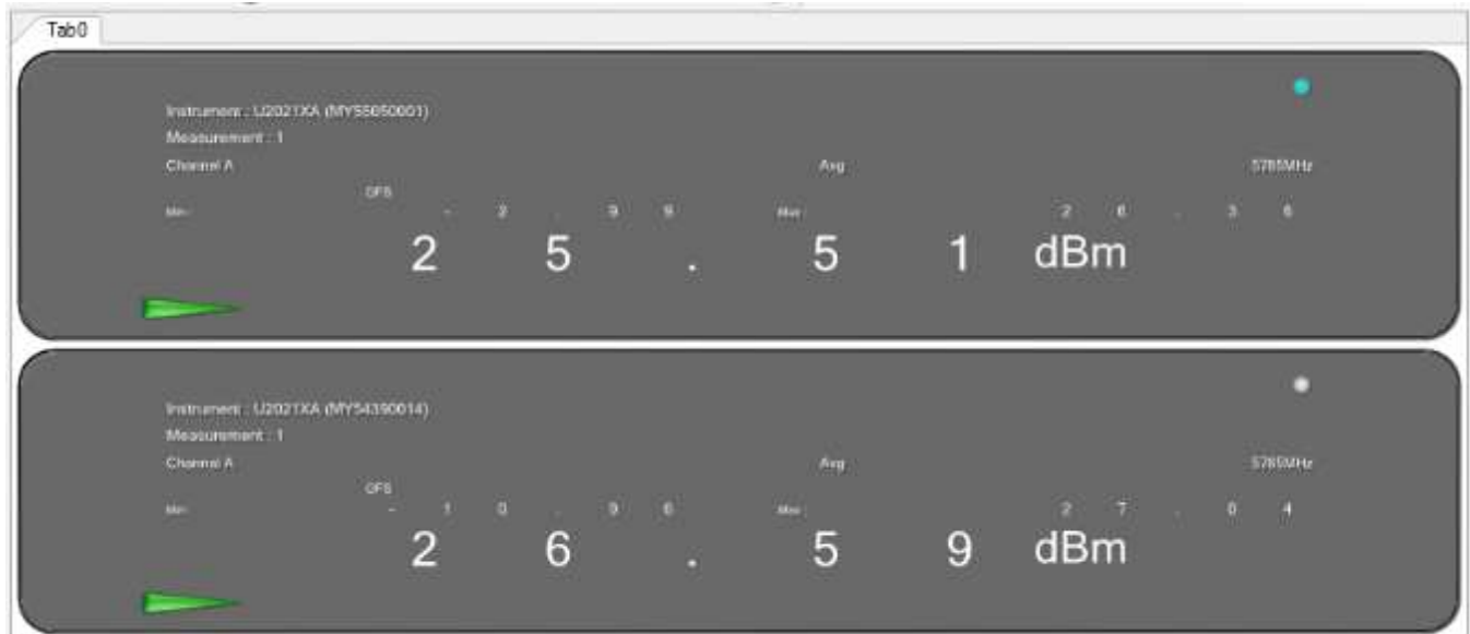
Figure 342: Maximum Conducted Output power measured at Ch.0 & Ch.1
