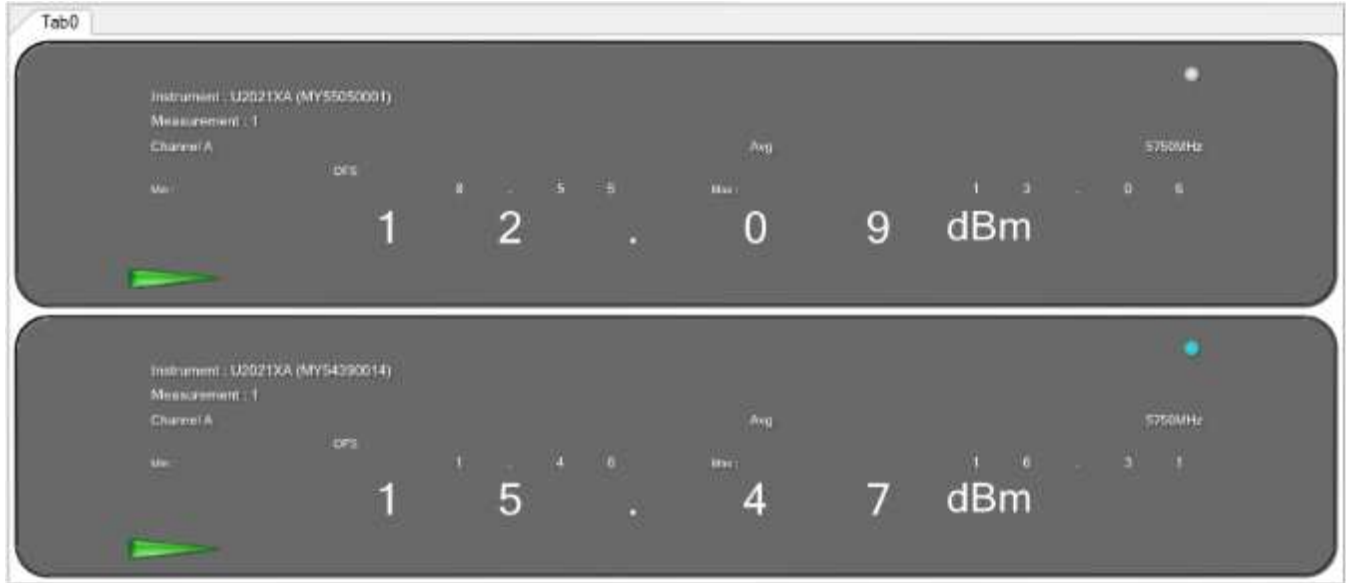
Figure 347: Maximum Conducted Output power measured at Ch.0 & Ch.1
