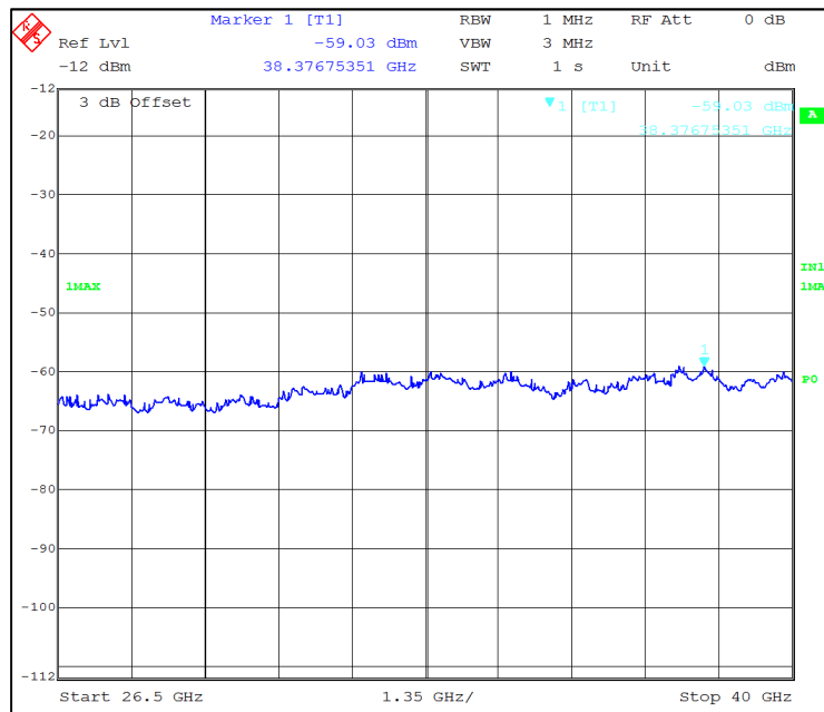
Figure 200: Emission measured with Peak Detector from 26.5GHz to 40GHz at Ch. 1
