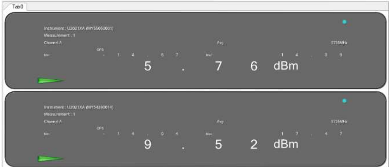
Figure 356: Maximum Conducted Output power measured at Ch.0 & Ch.1
