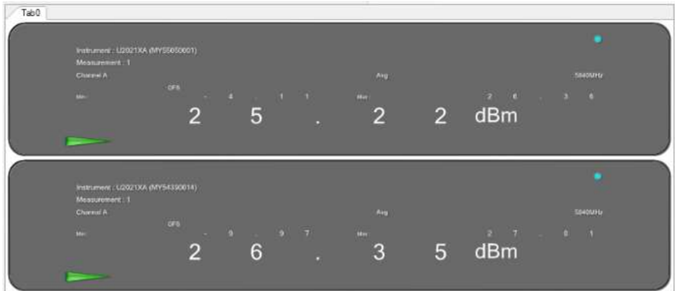
Figure 346: Maximum Conducted Output power measured at Ch.0 & Ch.1
