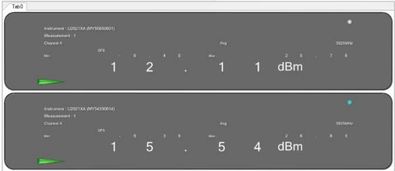
Figure 349: Maximum Conducted Output power measured at Ch.0 & Ch.1
