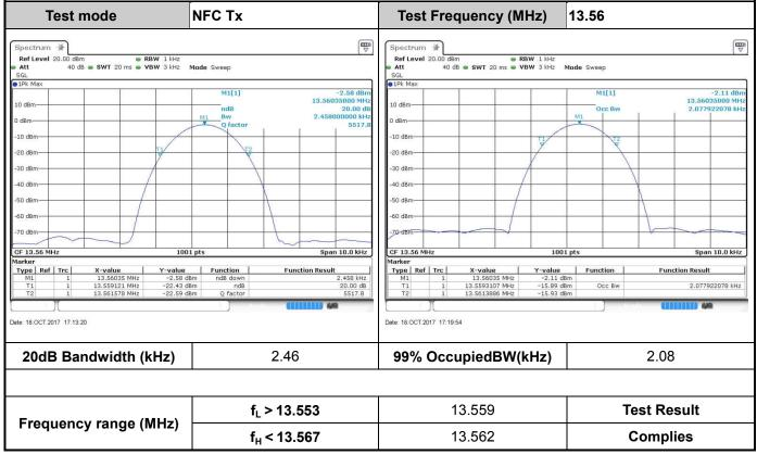
**Remark:** Because the measured signal is CW/CW-like adjusting the RBW per C63.10 would not be practical since measured bandwidth will always follow the RBW and the result will be approximately twice the RBW
