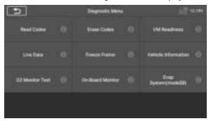
Figure 4-9 Sample OBDII Diagnostic Menu
