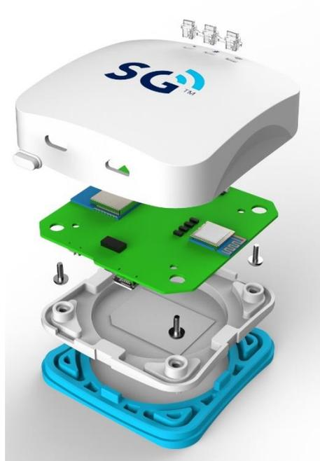
Figure 3. Internal Structure of SGW6008
