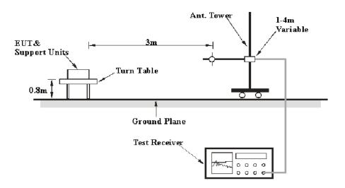
The radiated emission tests were performed in the 3 meters, using the setup accordance with the ANSI C63.10-2013. The specification used was the FCC 15.209 and FCC 15.247 & RSS-247/RSS-Gen limits.
