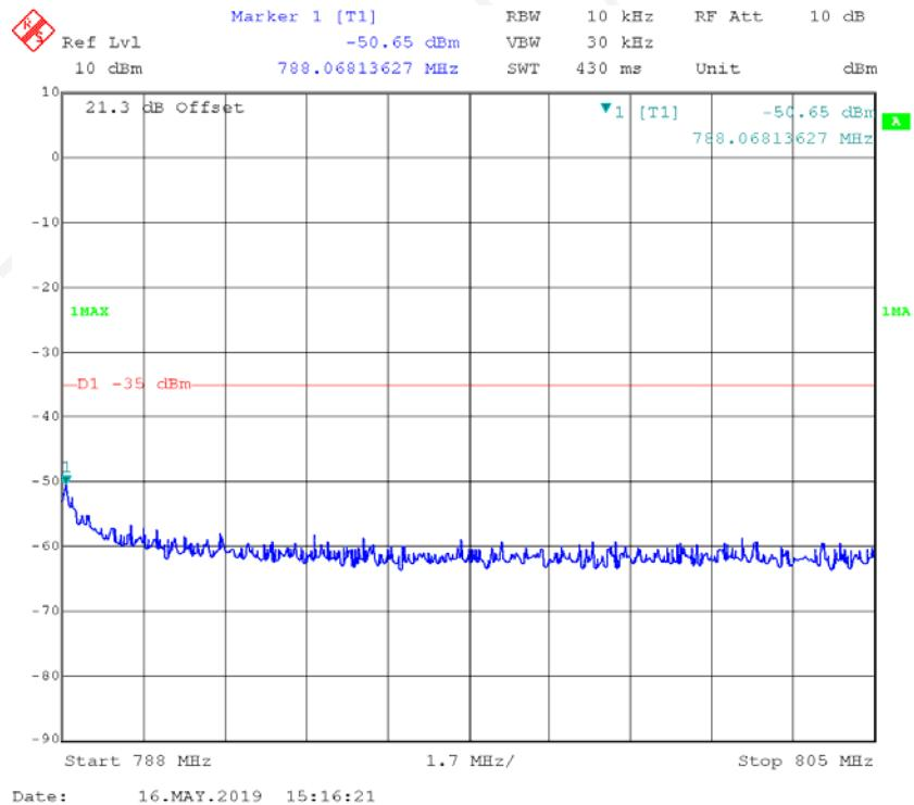
**FFSK1200, High power:****Channel Spacing 12.5 kHz, 787.5MHz**
