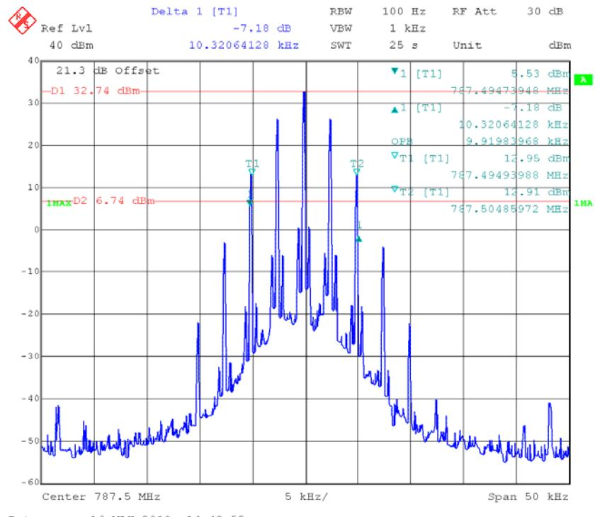
**FM,12.5kHz,Low Power - Frequency 787.5 MHz: 99% Occupied & 26 dB Bandwidth**
