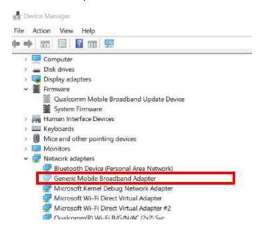
Wait around 120s Generic Mobile Broadband Adapter will back to normal device and then please reboot PC. During firmware update, you can find red led on and green led blinking.
