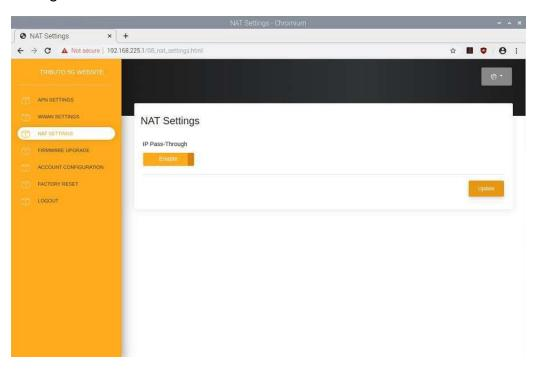
Dongle will reboot after enabled IP pass-through.
