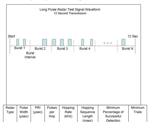
For the Frequency Hopping Radar Type, the same *Burst* parameters are used for each waveform. The hopping sequence is different for each waveform and a 100-length segment is selected<sup>1</sup> from the hopping sequence defined by the following algorithm:
