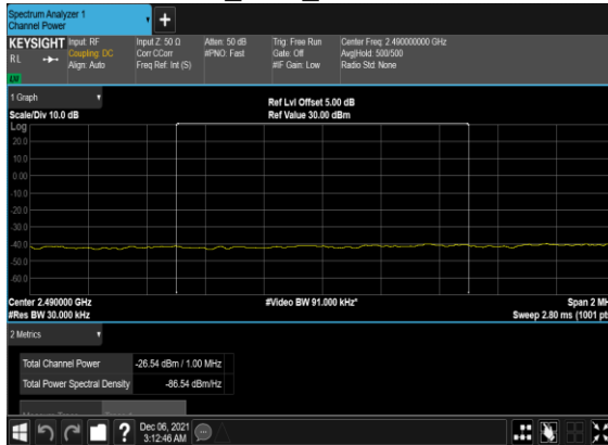
N7(20M)_DFT-s- OFDM_QPSK_Outer_Full_Low_CH CHP_PASS
