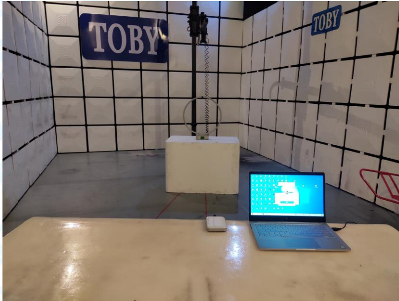
Photo of Setup for Radiated Emission (9KHz-30MHz)
