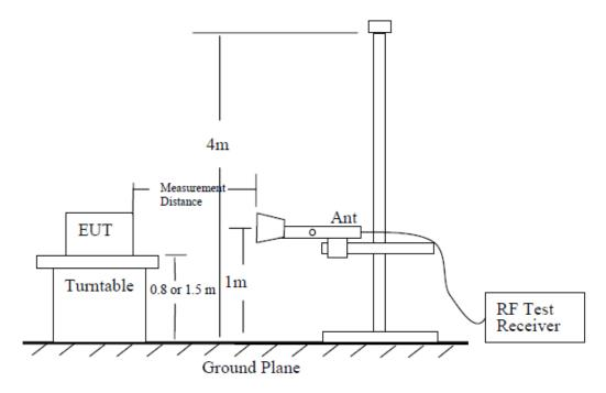
The emission characteristics of the EUT can be identified from the pre-scan measurement information.
