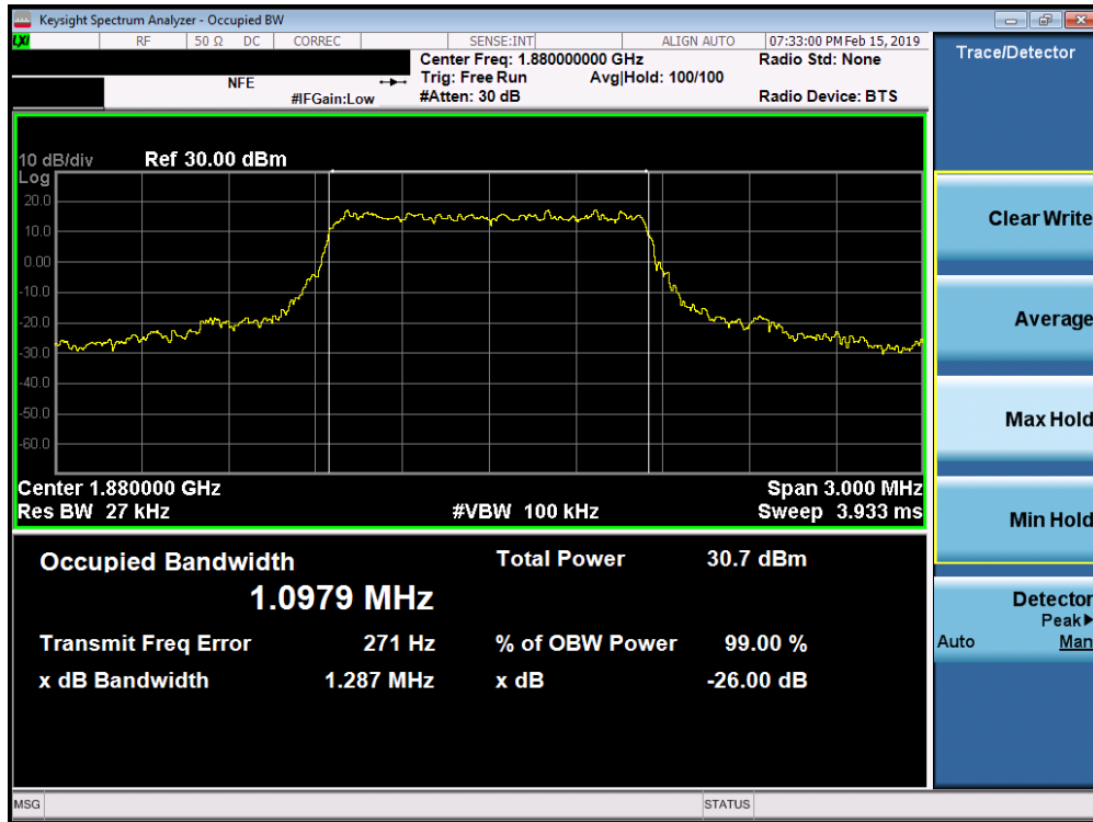
Plot 7-39. Occupied Bandwidth Plot (Band 25/2 - 1.4MHz QPSK - Full RB Configuration)
