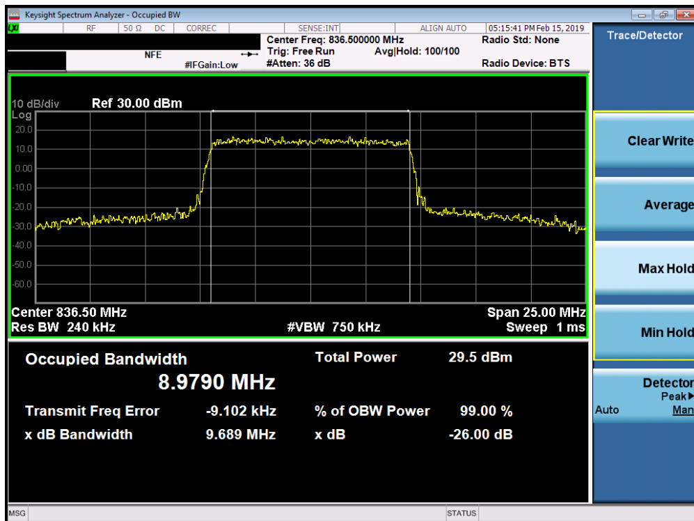
Plot 7-24. Occupied Bandwidth Plot (Band 26/5 - 10.0MHz 16-QAM - Full RB Configuration)
