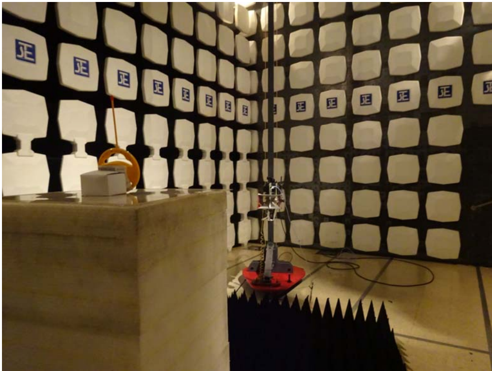
Measurement of Radiated Emission Test Set Up
