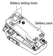
1. Push both battery sliding locks in the direction of the arrow. (1) The battery pack is then released.
