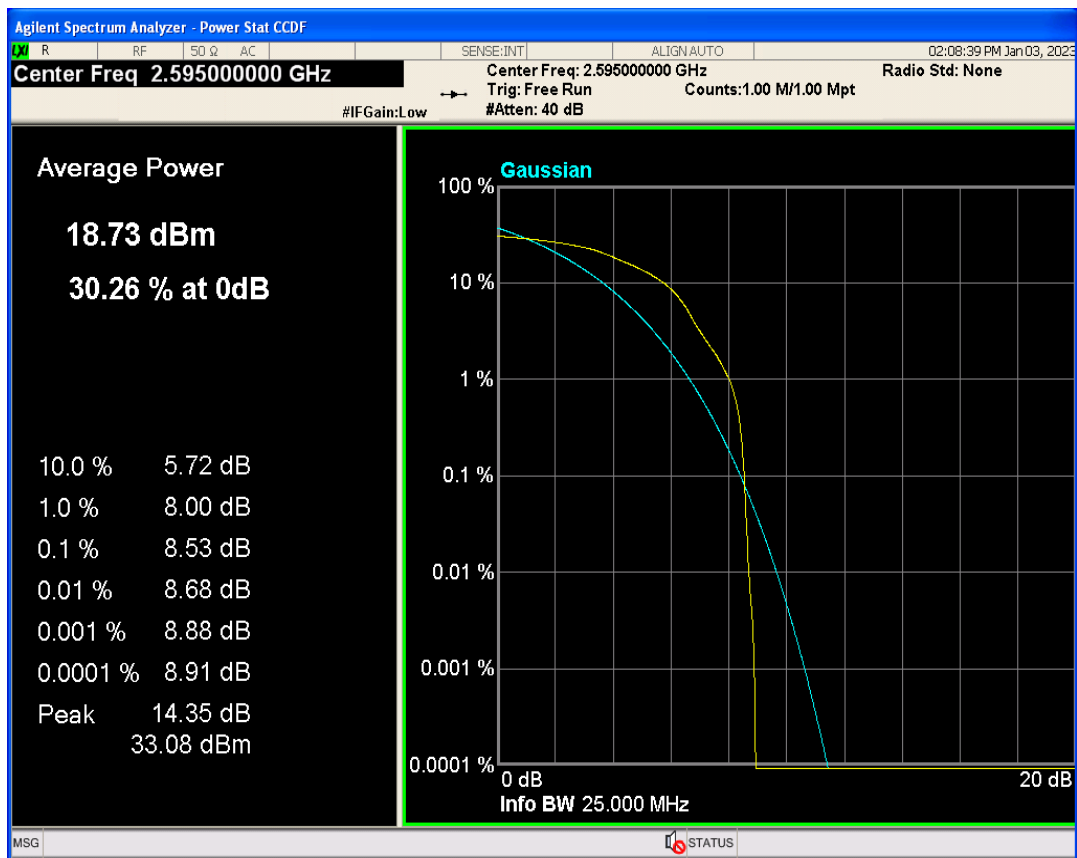
Band41 QPSK BW=10MHz Channel=40640 RB Size=1 Position=#0
