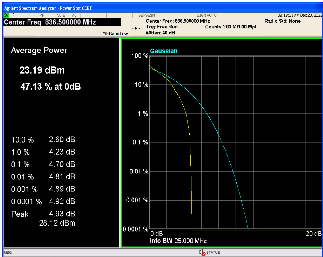
Band5 QAM16 BW=10MHz Channel=20525 RB Size=1 Position=#0
