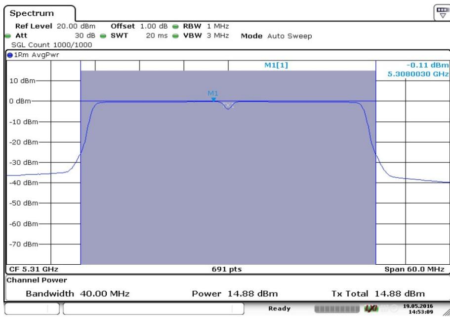
Radio Technology = WLAN n 20 MHz, Operating Frequency = mid, Subband = U-NII-2A
