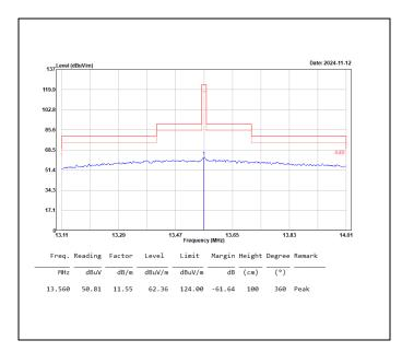
Level = Reading + Factor. Margin = Level – Limit. Factor = Antenna Factor + Cable Loss – Amplifier Gain.
