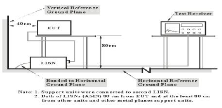
The setup of EUT is according with per ANSI C63.10-2013 measurement procedure. The specification used was with the FCC Part 15.207 and RSS-GEN limits.
