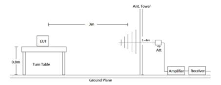
Radiated emission tests were performed in the 3 meters chamber test site, using the setup accordance with the ANSI C63.10-2013.
