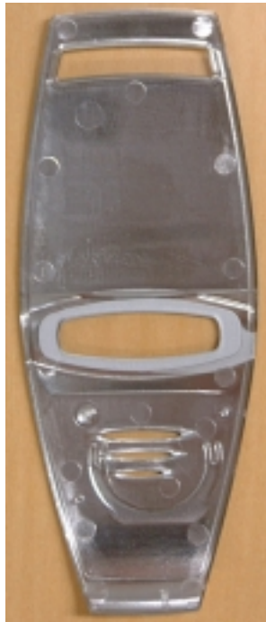
Metalized area of the front panel (back side view)
