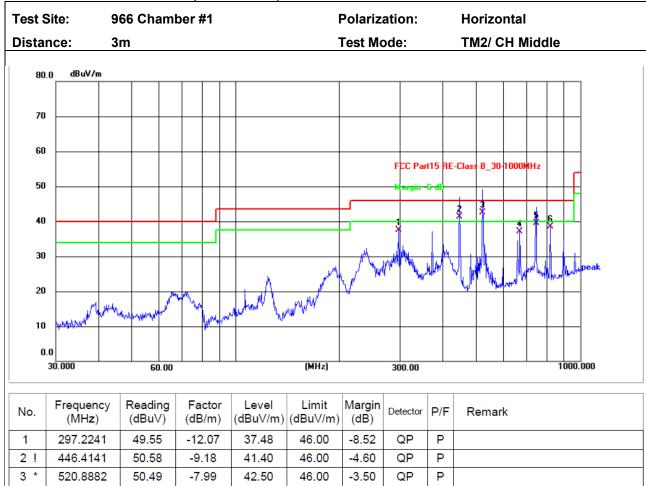
Note: Level = Reading + Factor Margin = Level - Limit
