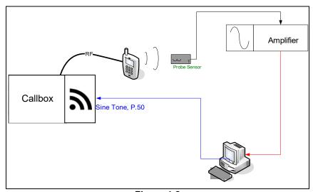
Figure 4-2 T-Coil Test Setup
