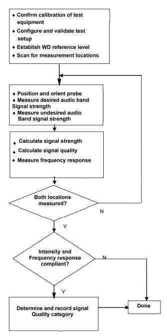
Figure 4-14 C63.19 T-Coil Signal Test Process
