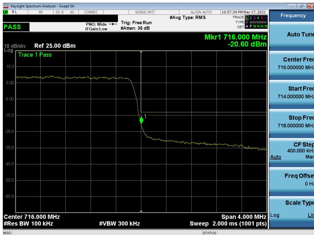
Plot 7-99. Upper Band Edge Plot (LTE Band 12 - 3MHz QPSK – Full RB)
