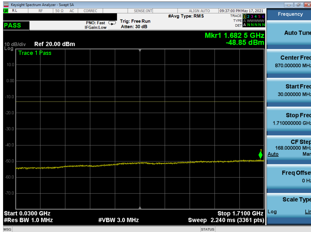
Plot 7-36. Conducted Spurious Plot (LTE Band 4 - 20MHz QPSK - 1 RB - High Channel)
