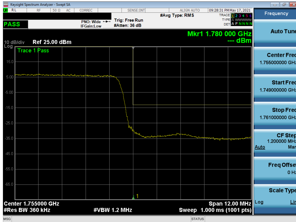
Plot 7-72. Upper Band Edge Plot (LTE Band 4 - 15MHz QPSK – Full RB)
