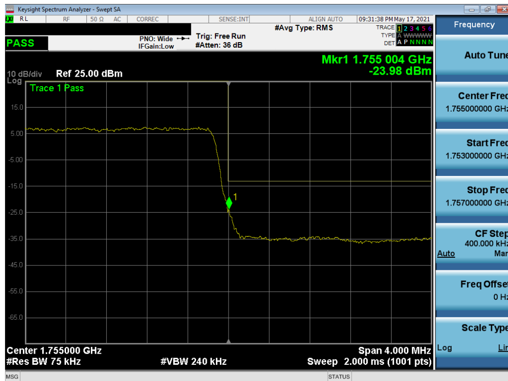
Plot 7-84. Upper Band Edge Plot (LTE Band 4 - 3MHz QPSK – Full RB)
