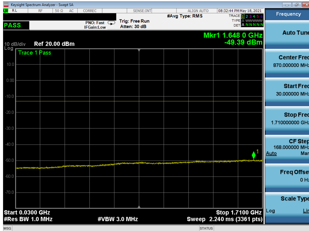
Plot 7-63. Conducted Spurious Plot (WCDMA Ch. 1513- High Channel)
