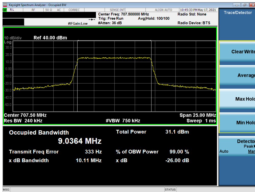
Plot 7-17. Occupied Bandwidth Plot (LTE Band 12 - 10MHz QPSK - Full RB)
