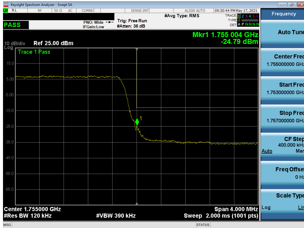
Plot 7-80. Upper Band Edge Plot (LTE Band 4 - 5MHz QPSK – Full RB)
