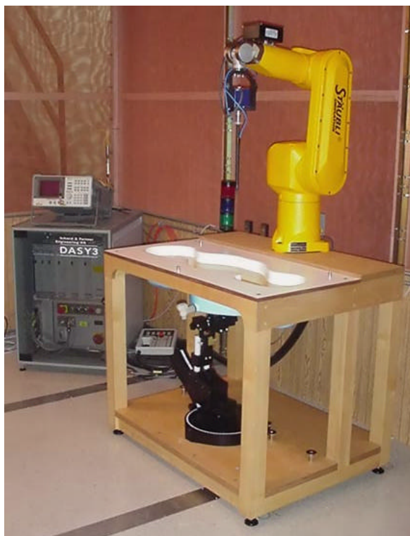
DASY3 SAR Measurement System
