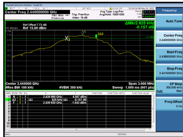
GFSK (BLE 1Mbps) MIDDLE CHANNEL
