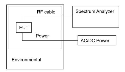
Note1:The frequency stability is measured with the temperature variation range of -20°C to +45°C, and voltage supply variation range of 85% to 115% of nominal AC supply voltage.
