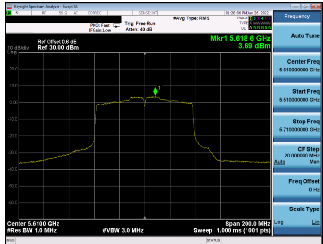
Plot 7-179. PSD Antenna WF8 (80MHz BW 802.11ac – Ch. 122, MCS3)
