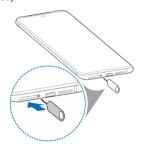
Pull out the card tray. You can place a nano-SIM card on the upper card slot, and place a microSDXC card (optional) on the lower card slot, as shown. Carefully slide the tray back into place.
