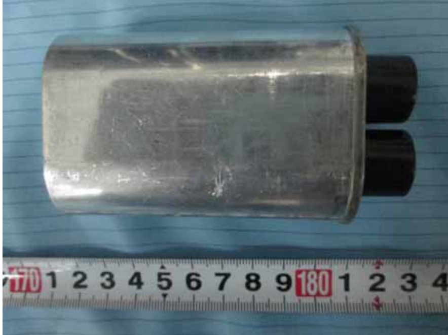
EUT – H.V. Capacitor Rear View
