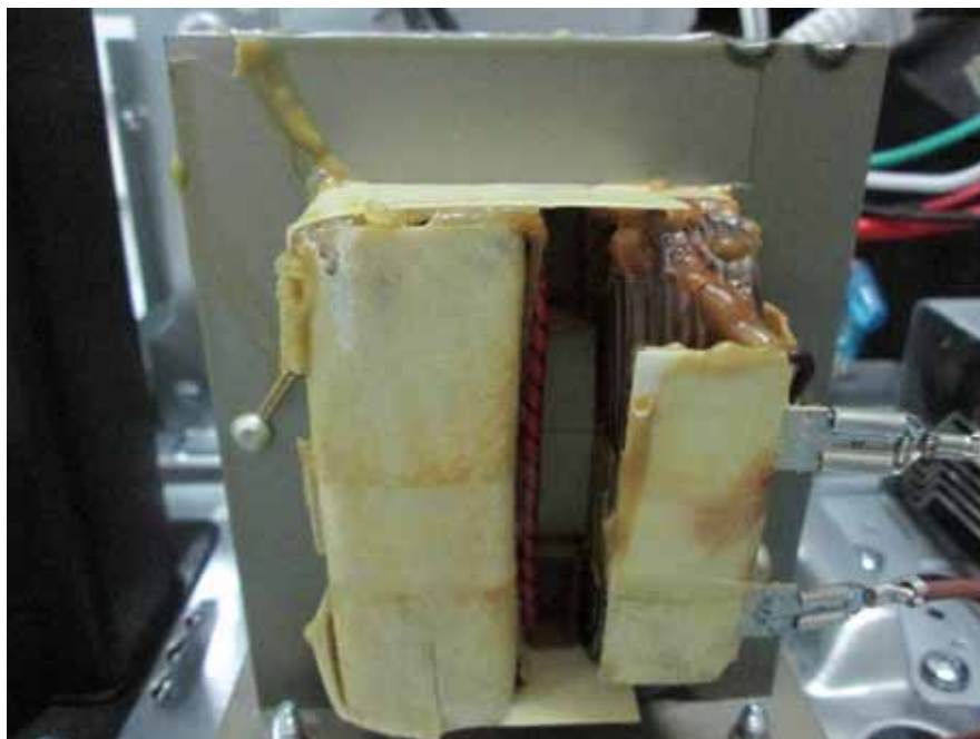
EUT – Power Transformer View
