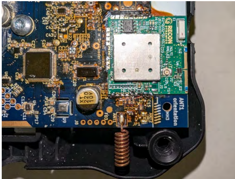
Photograph 57: View of Front of Module in the Host PCB and the RF Circuitry of the Wire-Wound Internal 900MHz Antenna
