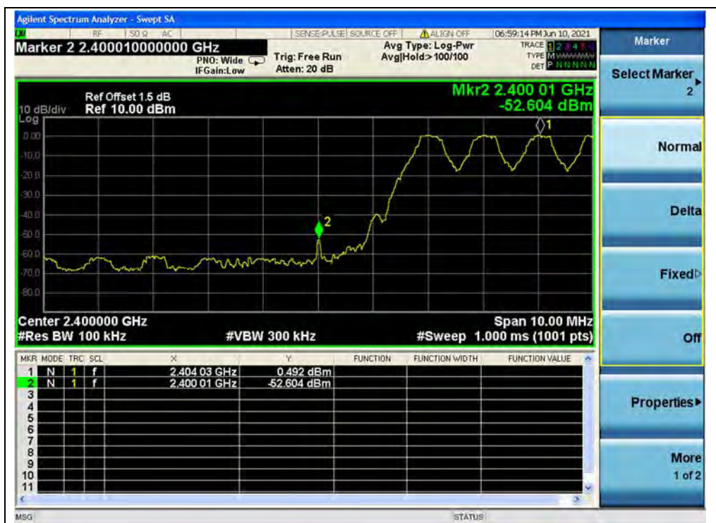
(Band edge with hopping on, Channel 0, GFSK)
