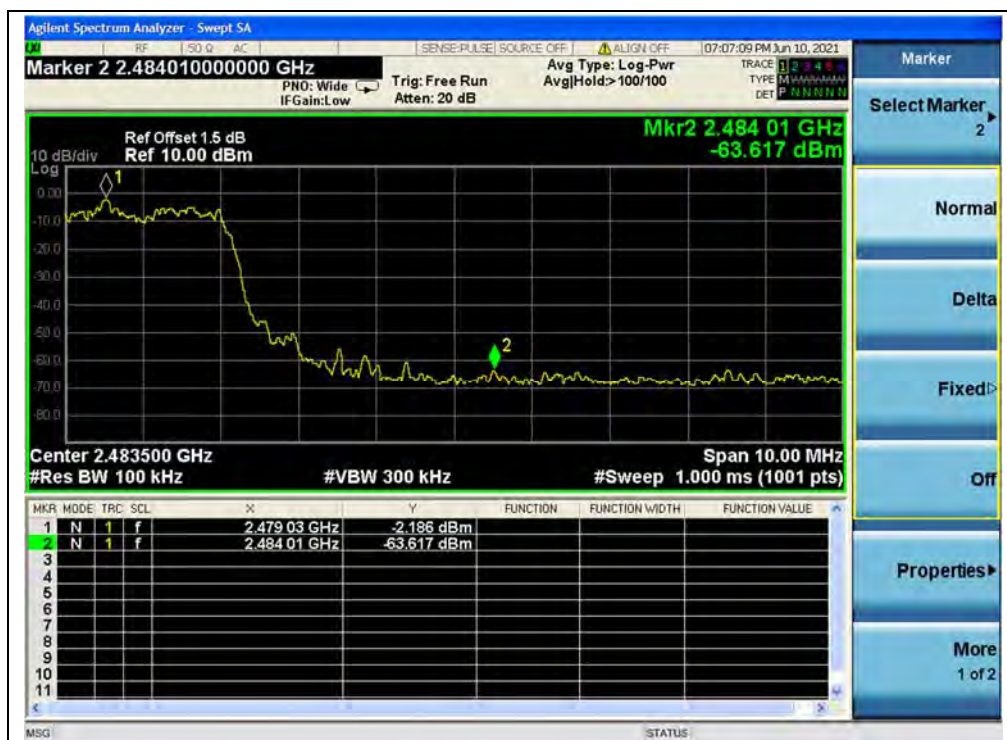
(Band edge with hopping on, Channel 78, 8-DPSK)
