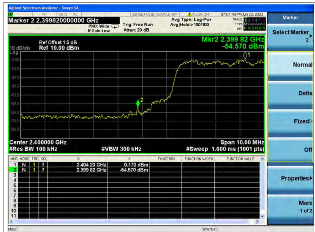
(Band edge with hopping on, Channel 0, 8-DPSK)
