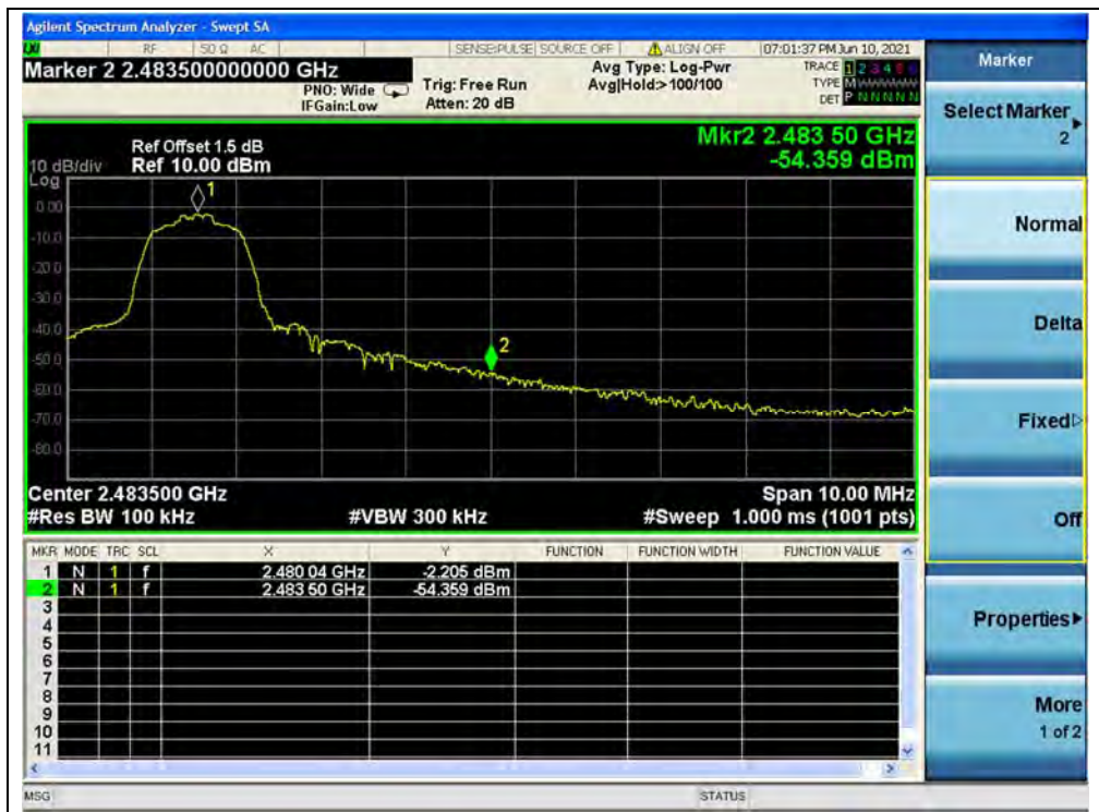
(Band edge, Channel 78, \pi/4 -DQPSK)
