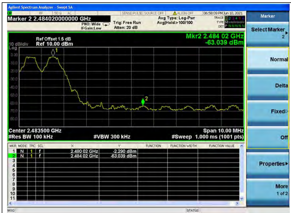
(Band edge with hopping on, Channel 78, GFSK)
