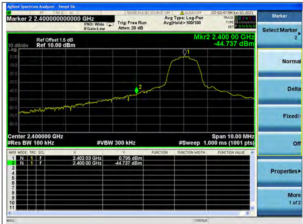
(Band edge, Channel 0, \pi/4 -DQPSK)
