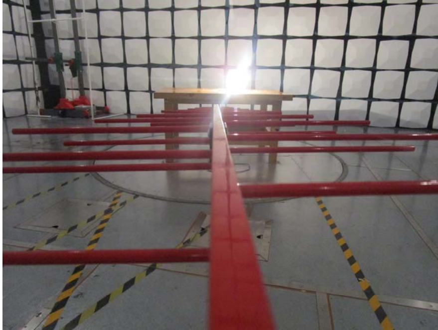
Radiated Emission View (Below 1GHz)
